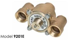
AXION thermostatic mixing valve that mixes hot and cold water to supply tempered water to emergency shower and eyewash fixtures requiring flow up to 31 GPM (117 LPM). CSA Certified to ASSE 1071 and applicable sections of CSA B125.3.
