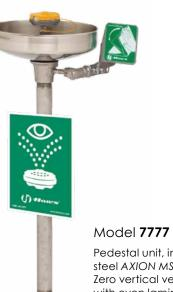
Pedestal unit, includes a Type 304 stainless steel AXION MSR eve/face wash head. Zero vertical velocity™ stream engineering with even laminar flow. Features a round 11" (28 cm) Type 304 stainless steel receptor, and 1-1/4" (3.175 cm) stainless stanchion. Optional stainless steel dust cover, model 9102.
